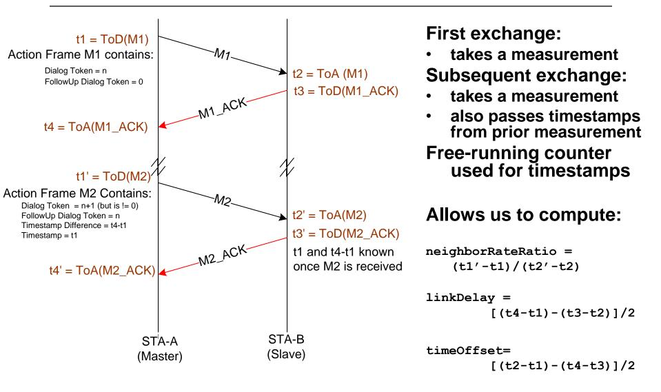
NOTE: M1 and M2 have exactly the same format they're TIMINGMSMT Private Action Frames (and Unicast, BTW) [note: rateRatio is also applied]
