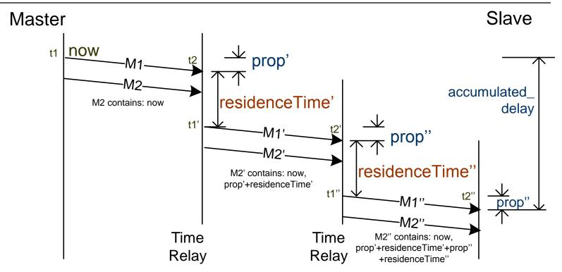
Grand Master initiates timing message, shown as M1, every Sync Interval At each hop, propagates *now* and measures the actual delay of M1:
