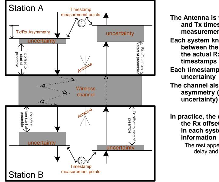
The Antenna is the *reference* for Rx and Tx timestamp measurements
