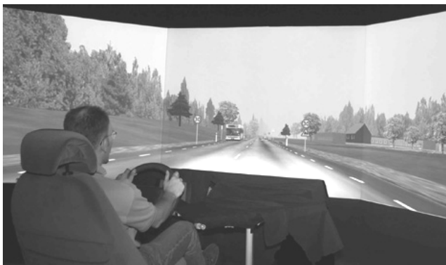
Figure 2: The driving simulator that is used in our study. The simulator is a fixed-based, software-oriented system, which allows for rapid prototyping of new support systems to be tested.
