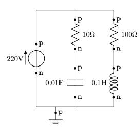
$$\begin{aligned} u &= A \cdot sin(\omega t) \\ u_3 &= R_2 \cdot i_2 \\ u_1 &= u - u_2 \\ u_4 &= u - u_3 \\ i_1 &= \frac{u_1}{R_1} \\ i &= i_1 + i_2 \\ \dot{u}_2 &= \frac{i_1}{C} \\ \dot{i}_2 &= \frac{u_4}{L} \end{aligned}$$
