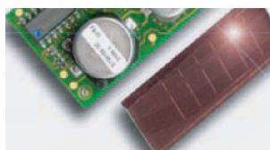
Solar cell, can operate several days in darkness, sleep mode ~25 nA
