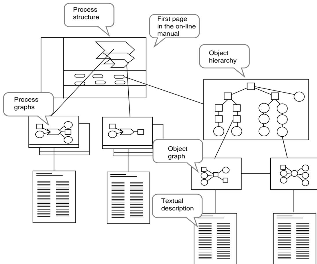
**Figure A** A schematic picture of the on-line manual. The two overview pictures show the process structure and the object hierarchy. From those, each process and object description can be reached.
