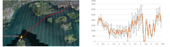
(a) Commuter path (b) B/w variation Fig. 4: Ferry scenario (5.9 km over 9 min 52 sec).
