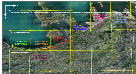
Fig. 2: Network performance map for the bus scenario (cf. Section IV-A) with 1000m resolution.
