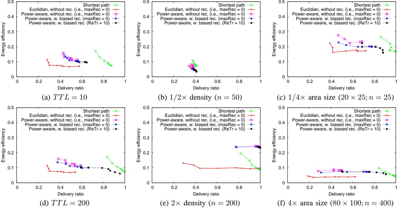
Fig. 6. Policy comparisons for a number example scenarios. The impact of  $TTL$  is illustrated by (a) and (d). The impact of the node density is illustrated by (b) and (e). The impact of the network size is illustrated by (c) and (f). (Default scenario:  $n = 100$ , size= $40 \times 50$ ,  $TTL = 50$ ,  $f = 0.5$ .)
