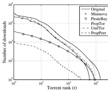
Fig. 8. Rank popularity statistics for five methods of sampling the measured number of downloads in 4 weeks starting on 15 Sept. 2008.
