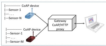
**Figure 1: An example architecture of Web services in WoT environments.**
