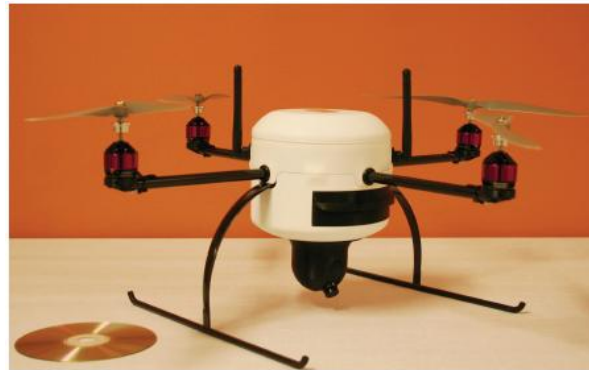
LinkQuad weight ~1 kg, diameter ~70cm
