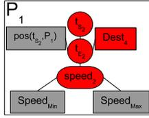
Figure 3: The parameterized platform constraints for the scan action. The red/dark variables are connected to the TST as part of the node interface.
