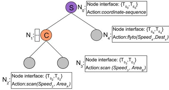
**Figure 1: An example TST for first scanning Area<sub>A</sub> and Area<sub>B</sub> concurrently and then flying to Dest<sub>4</sub>.**
