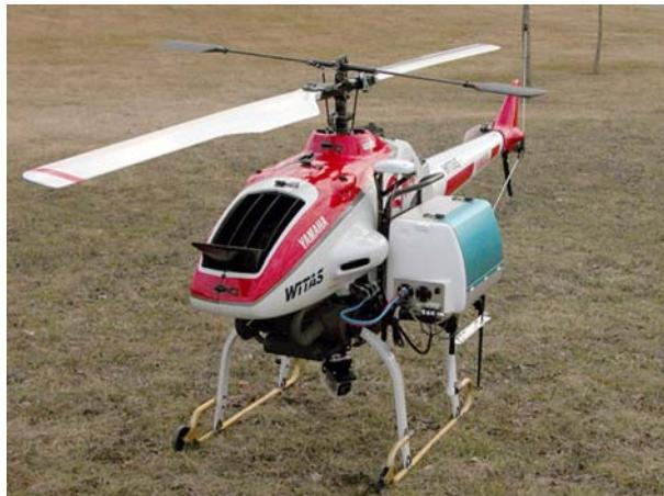
**Fig. 1** The UASTech Yamaha RMAX helicopter
