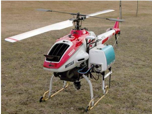
**Fig. 1** The UASTech Yamaha RMAX helicopter
