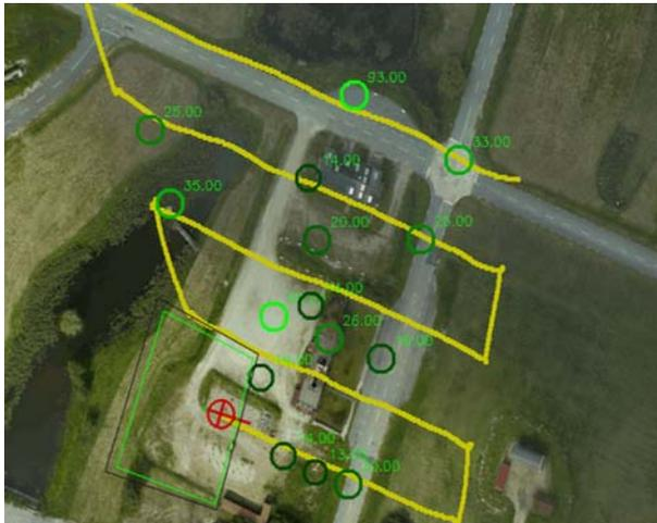
**Fig. 9** Flight path and geolocated body positions
