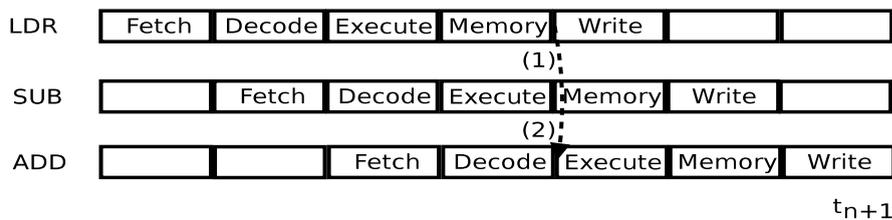
The data for R3 enters LDR's memory stage (1) before it is used by ADD's execution stage (2). No processor stall is needed and this group of instructions takes just as long time to be processed as the two instructions in the first example.
