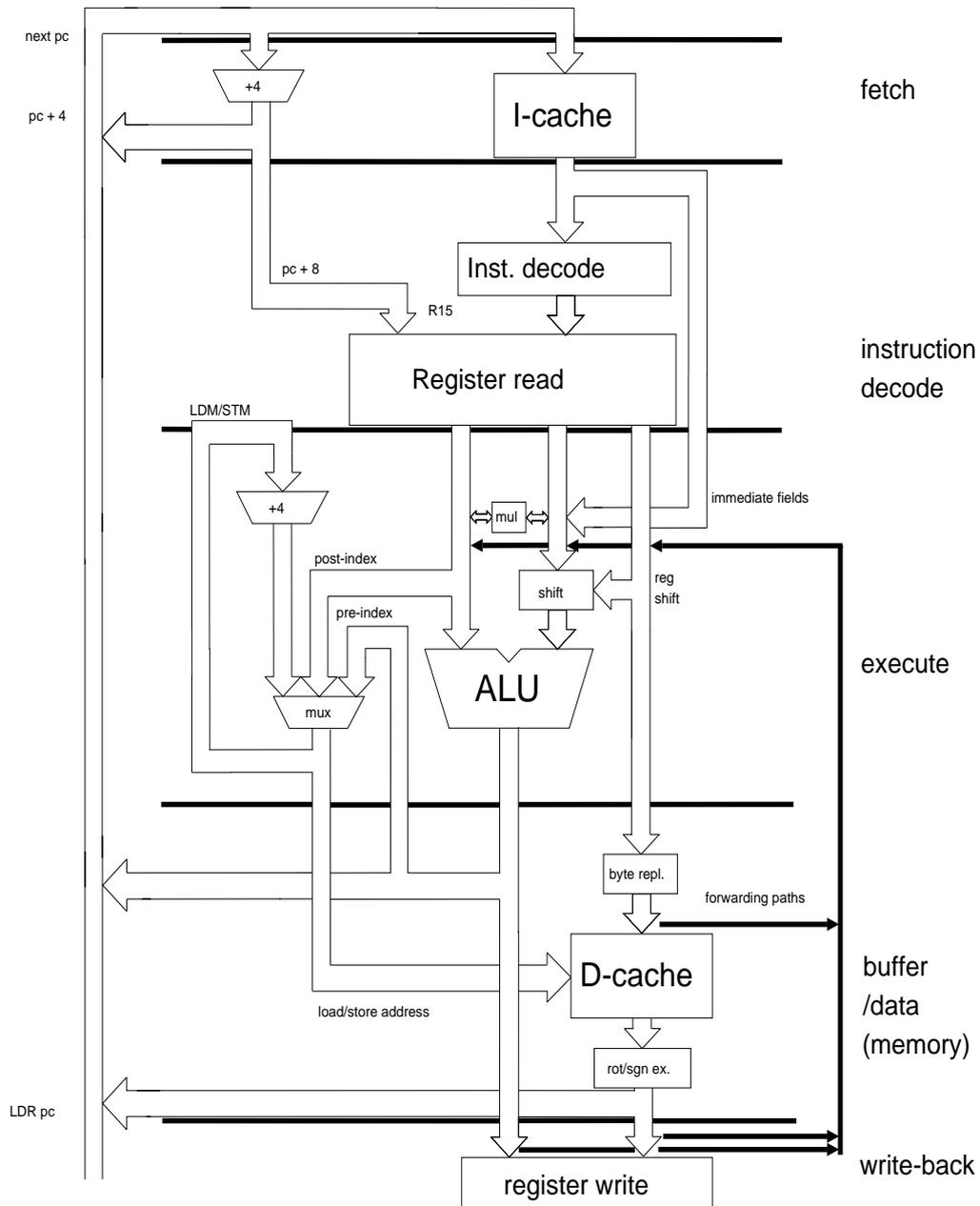
**Figure 4.2** The ARM9E processor core.
