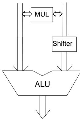
**Figure 5.1** The MUL, ALU and shifter unit in the ARM9E processor.
