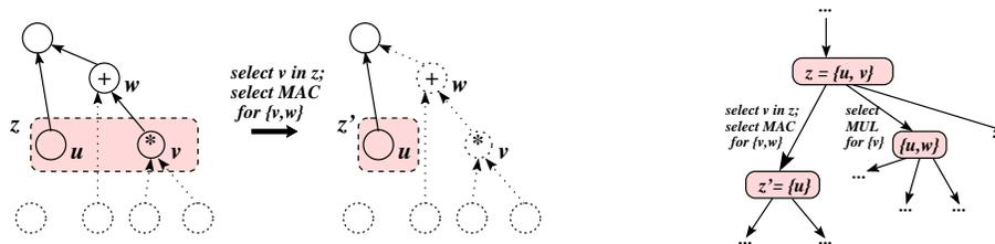
Figure 1: Basic method. Left hand side: situation when selecting  $v \in z$  and a multiply-accumulate instruction that covers  $v$ . Right hand side: resulting selection tree.
