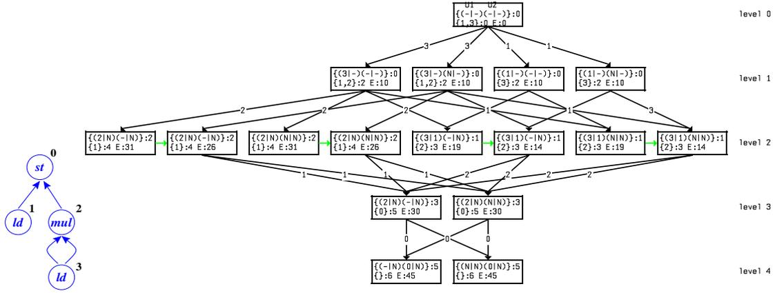
Figure 2: Solution space for squaring on a 2-issue architecture with 2 functional units  $\ell = (2, 1)$ , with base costs: 4 for st, 3 for others, 1 for NOP, and instruction overhead of 0.
