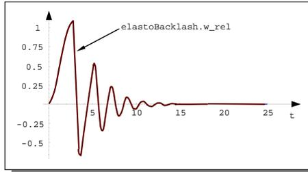
Relative rotational speed between the flanges of the Elastobacklash transmission
