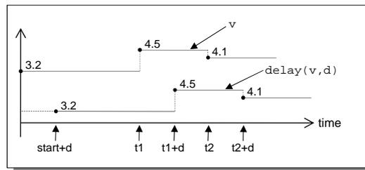
In the expression `delay(v, d)` `v` is delayed by a delay time `d`
