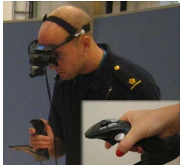
Figure 3: The redesigned interaction device, which allows the user to choose a virtual object and place it on the digital map.
