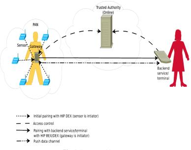
Fig. 1. System architecture
