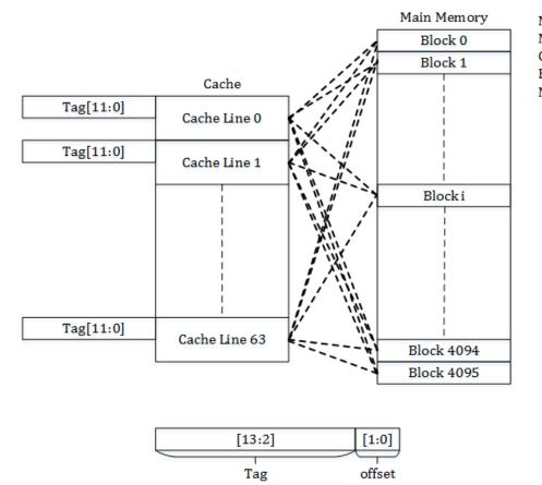
Memory Size = 16Kbytes Memory Block Size = 4 bytes Cache Size = 256 bytes Block Size = 4 bytes Number of Cache Lines = 64
