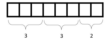
Consider a machine with a byte addressable main memory of 2^8 bytes and block size of 4 bytes. Assume that a direct mapped cache consisting of 8 lines is used with this machine.
