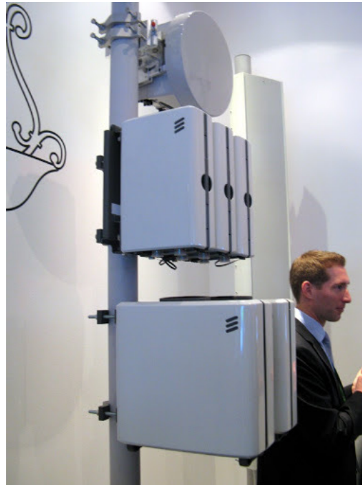
Ericsson RBS 6302 Weight of RRU is 20 kg Main cabinet – 70 kg
