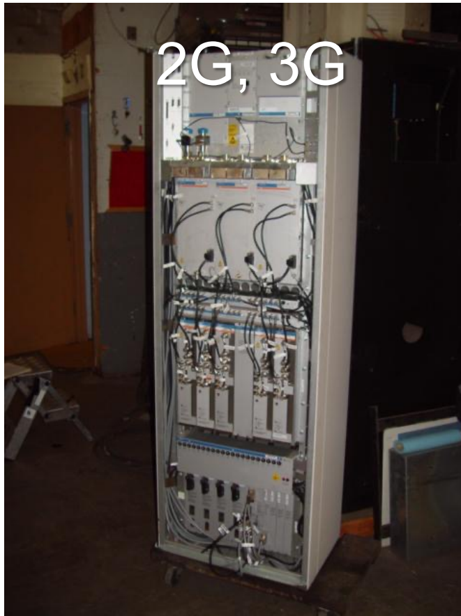
Ericsson RBS 2206 – max 12TRXs (3x4) Fully equipped cabinet – 230 kg
