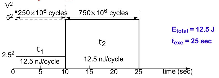
If power consumption per cycle differs from task to task the "basic principle" is no longer true!
