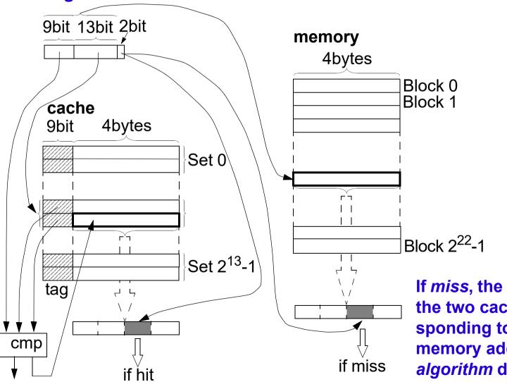
If *miss*, the block is placed in one of the two cache lines in the set corresponding to the 13 bits field in the memory address. The *replacement* algorithm decides which line to use.
