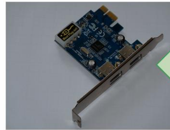
PCIe card with two USB 3.0 ports, 2013, photo courtesy of Dmitry G under public domain
