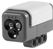
Figure 8: "The Colour Sensor can distinguish between colours and also works as a Light Sensor, detecting light settings and ambient light, and works like a lamp, shining red, green or blue"
