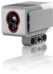
Figure 8: "The Colour Sensor can distinguish between colours and also works as a Light Sensor, detecting light settings and ambient light, and works like a lamp, shining red, green or blue"
