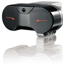
Figure 9: "The digital EV3 IR Seeker Sensor detects/measures proximity to the robot and reads signals emitted by the EV3 IR Beacon."
