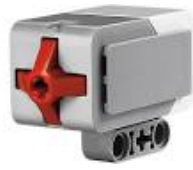
Figure 7: "The Touch Sensor makes your robot "feel" so that it can react to its environment"
