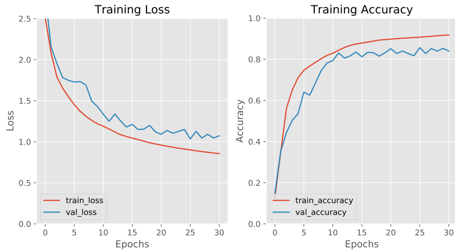
Figure 3.2: Loss over epochs, training accuracy and validation accuracy for Segnet on the Camvid dataset.
