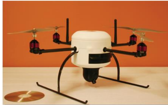
LinkQuad weight ~1 kg, diameter ~70cm
