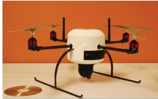
LinkQuad weight ~1 kg, diameter ~70cm
