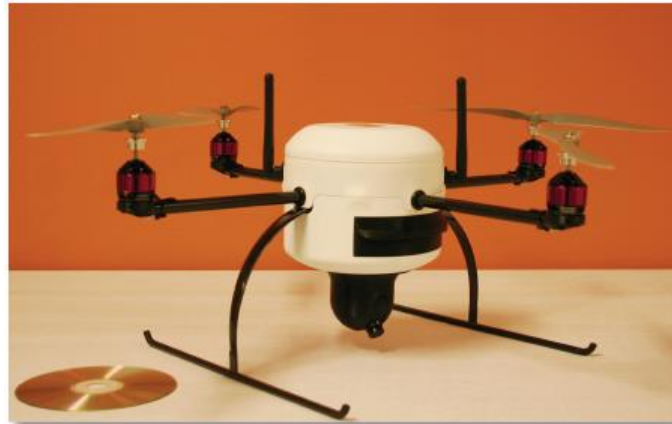
LinkQuad weight ~1 kg, diameter ~70cm
