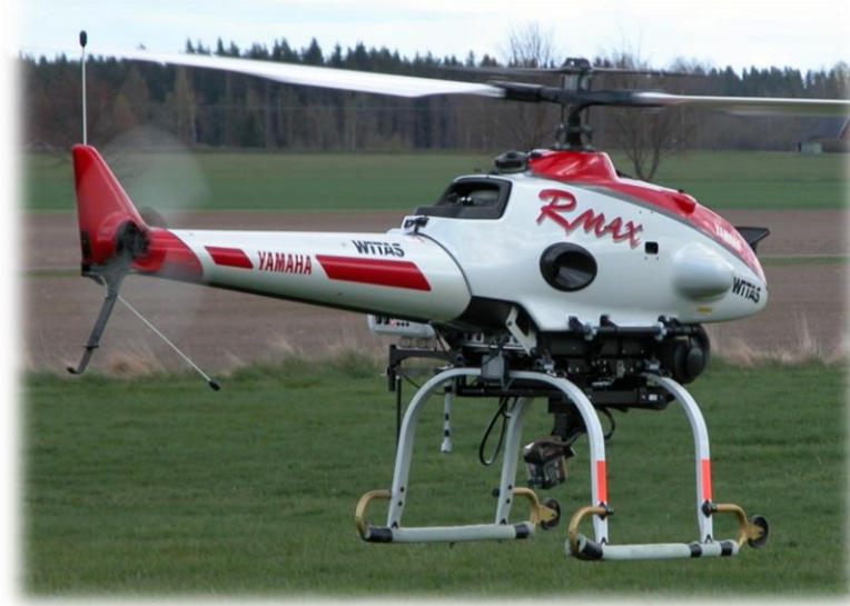
Yamaha RMAX weight 95 kg, length 3.6 m
