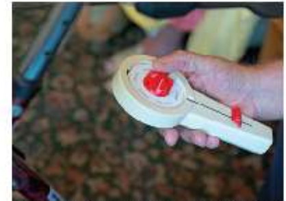
The wireless controller tunes into different categories of photographs and controls how far the topic may drift.
