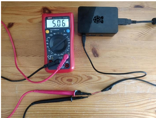
Figure 2: Setup for measuring the voltage
