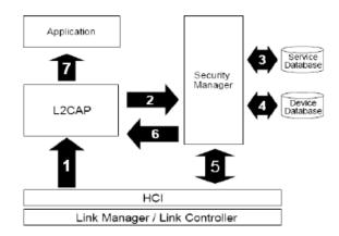
Regarding the protocol stack, for any new connection request, the request submitted to L2CAP, in some cases also in RFCOMM for multiplexing, and then the protocol parameters are passed to the security manager for decision making. These parameters enter as query values to the security manager. Finally, the security manager according to it is query results; may either grant access or reject the access.
