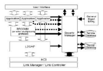
Bluetooth security architecture resides in L2CAP layer and above it. The only Bluetooth specific is RFCOMM, all other are not Bluetooth specific. L2CAP: enforce security for cordless telephony. RFCOMM: enforce security for Dial-up networking. OBEX: files transfer and synchronization. Establishing a connection (from the layers)
