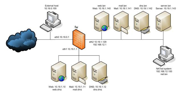
Each system has a separate UML instance with a single IP address. The appropriate services are configured (to some extent) on each of your servers. The web server is dhttpd, a small and very simple server; the mail server is Postfix; and the DNS server is BIND 9. All hosts use the internal DNS server to look up names.
