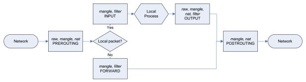
Built-in chains (PREROUTING, INPUT, OUTPUT, FORWARD, and POSTROUTING) also have a policy (user-defined chains do not), which is a target applied to any packet that reaches the end of the chain (because no classifier matched, or because no target aborted processing of the chain).
