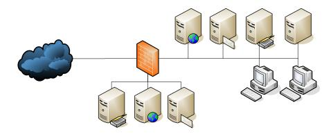
In this lab you will set up a Linux-based system as a firewall, according to a network security policy provided to you. The implementation will be done using a virtual Linux network designed to mimic a fairly typical corporate network scenario.
