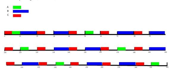
You can try to change the order of execution of the tasks, but the jitter still remains. One of the possible ways to schedule this task set without jitter is by reducing the periods, thus executing tasks more frequently than required (see Example (3.2), i.e. Alternative 2 in the slides of Lecture 2).
