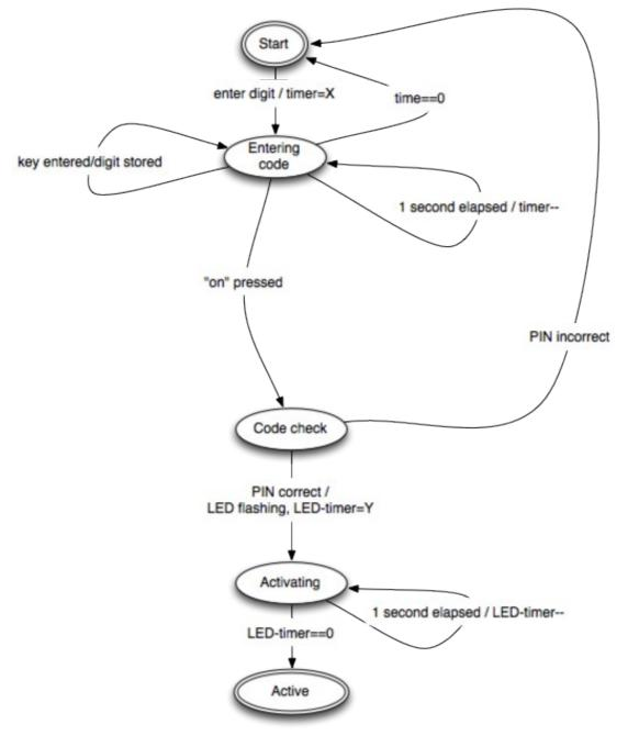
Such a state chart can be used to devise test cases for coverage of either the nodes, edges or paths in the graph.
