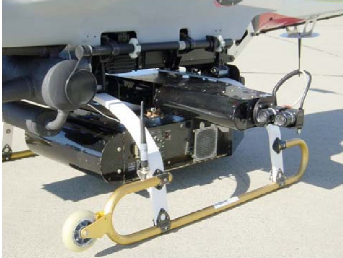
Stereo pair of 1m baseline – cross-shaft for stiffness
