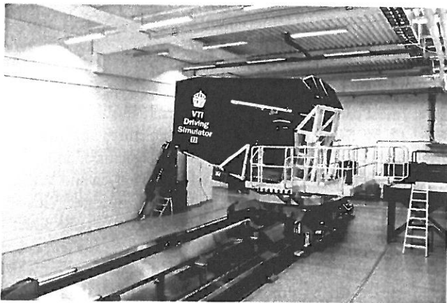
FIGURE 4.2 The VTI driving simulator in Linköping, Sweden. This also is one of the most advanced, state-of-the-art motion-based driving simulators in the world. (Photograph: P.A. Hancock, reproduced by permission of VTI.)
