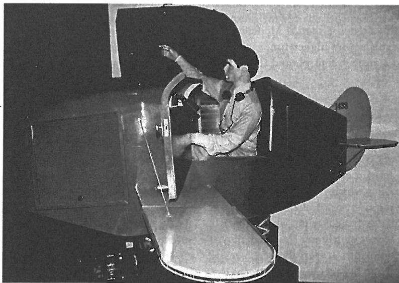
FIGURE 4.3 The original Link Trainer or "blue box" as it was affectionately known. Although there is no true motion base per se, the facility did sit on a platform which provided some movement.
