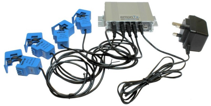
Figure 1: “Open Energy Monitor” metering device (Open 2016).
