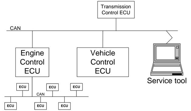
**Figure 1. An heterogeneous automotive control system**
