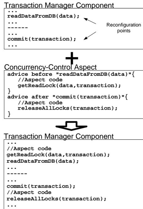
**Figure 5. A simplified example of the weaving process**
