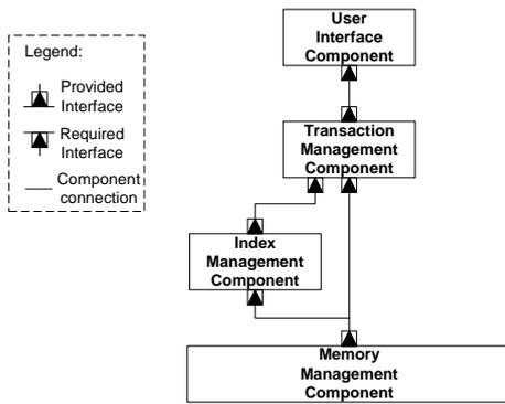
**Figure 3. The basic architecture of COMET**
