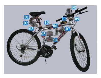
01 = mike 02 = magnetometer 03 = pedal speed 04 = inclinometer (tilt) 05 = sink with 802.15.4-to-Bluetooth interface 06 = lateral tilt 07 = Galvanic Skin Resistance Stress Monitor 08 = Mobile Phone 09 = Speedometer and odometer 10 = CO2 meter 11 = GPS
