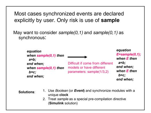
In **Simulink-like solution**, *samples* would be synchronized with each other by finding a fastest common clock. But they are not synchronized with other time events.
