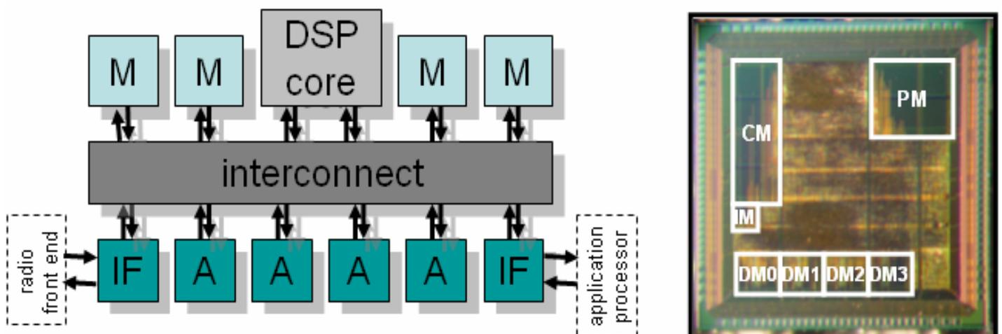
Figure 3. Programmable baseband processor architecture and prototype chip
