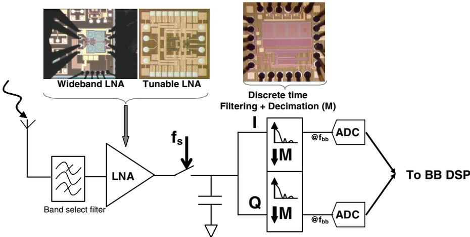
**Figure 1. RF-sampling front-end**
