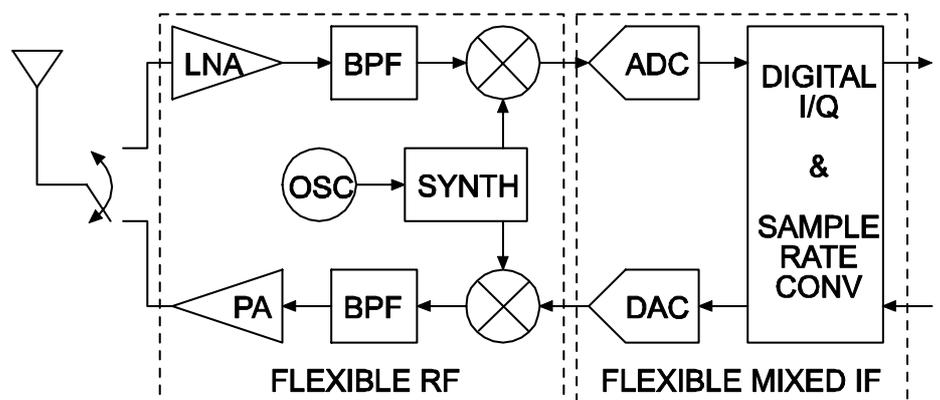
**Figure 2. Digital-IF transceiver with flexible RF and mixed-signal**
