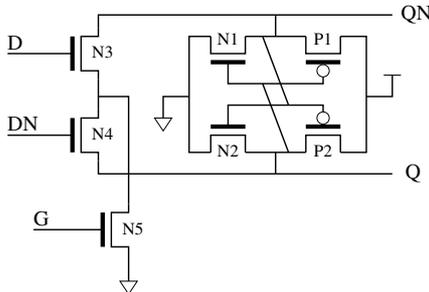
Figure 2: Static latch used in the data path.
