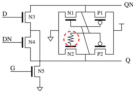
**Figure 6:** Schematic of a bit-cell with a resistive open at one of the NMOS transistor gates of the cross-coupled inverters.
