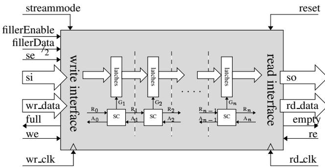
Figure 1: The architecture of the FIFO module.
