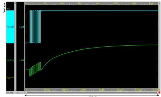
**Figure 7:** Voltage on the data line (upper curve) and on the broken gate connected to the same data line by a 1 GΩ resistance (lower curve).
