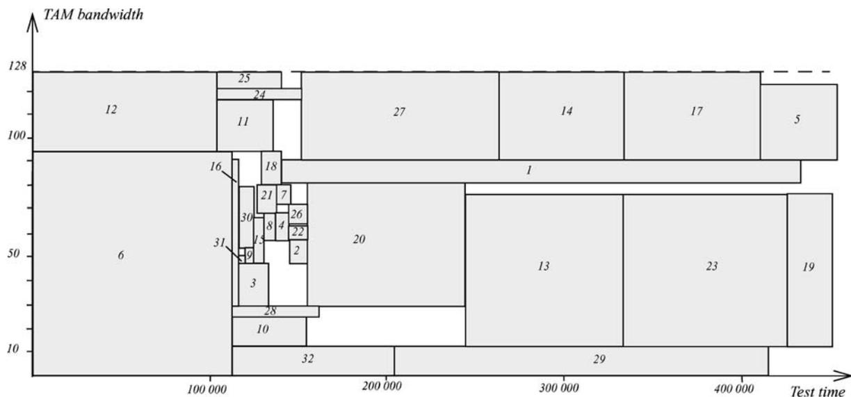
Fig. 10. Test schedule for p93791 with  $W_{\max} = 128$  bits.
