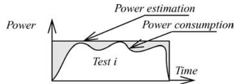
Fig. 3. Modelling of test power consumption.
