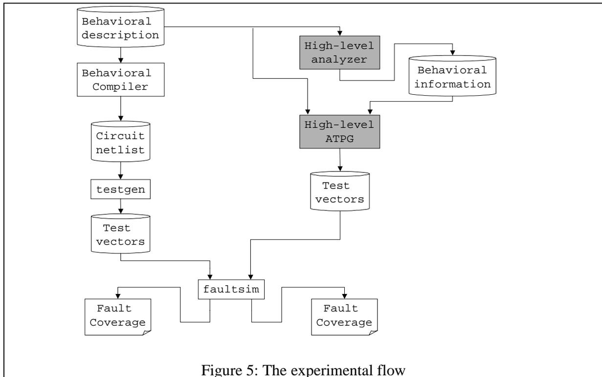
On the left-hand of Figure 5, the traditional approach to test vector generation is reported. Starting from a behavioral description of the circuit, the Behavioral Compiler tool by Synopsys will be used to generate a netlist implementing the desired behavior. Then, the Synopsys gate-level ATPG (testgen) will be used to compute a set of test vectors. Finally, the Synopsys fault simulator (faultsim) will be used to evaluate the attained fault coverage.
