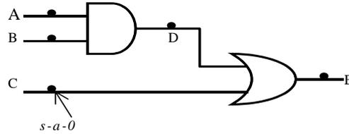
Figure 2.1 Single stuck-at faults
