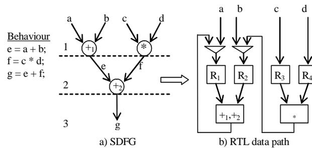
Figure 3.1 An SDFG and its corresponding RTL data path
