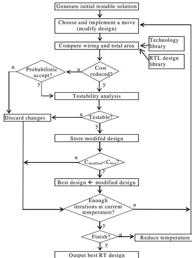
Figure 5.3 Simulated annealing BIST synthesis framework
