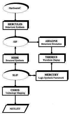
parallelism that exists in the input description. Here, the input HardwareC description is parsed and translated first into an abstract syntax tree representation, which provides the underlying model for semantic analysis and behavioral transformations. The transformations are categorized into user-driven and automatic transformations.
