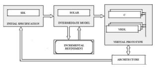
scheme, in a distributed model that matches with the architectural solutions. Each step reduces the gap between specification and realization by fixing some implementation details (communication protocol, generating software or hardware code) or by preparing future implementation steps (merging and scheduling several processes to execute them in a single processor).
