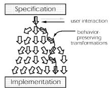
transformations from a designer defined hierarchical list of transformations. After the transformation, a SIL to VHDL Translator will generate the VHDL codes, which can be synthesized using commercial RT-level synthesis tools.
