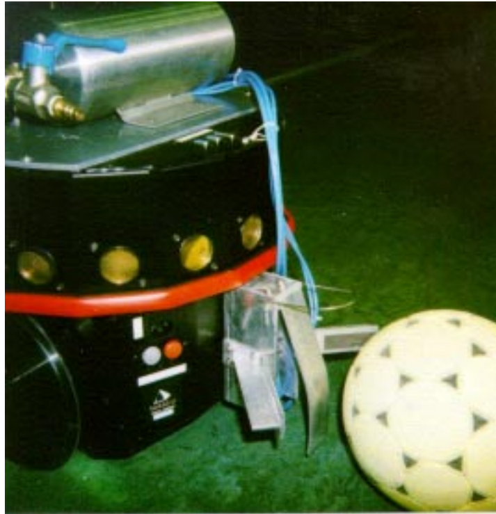
Figure 1: The Nomad autonomous robot with (prototype) kicking device
