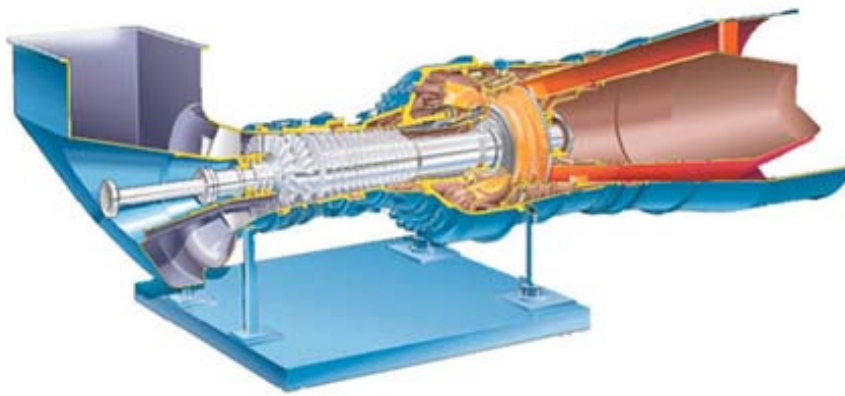
Figure 1-7. A schematic picture of the gas turbine GTX100. Courtesy Alstom Industrial Turbines AB, Finspång, Sweden.
