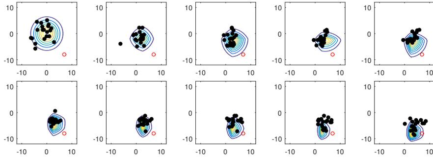
The black dots are the particles, the red circle is the true position of  $x_0$  and the contours are proportional to  $\pi_n$ , for  $n = 1, \dots, 10$ .
