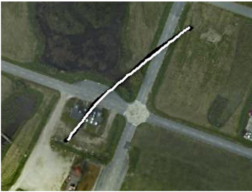
Fig. 6. Autonomous flight between two points over building. Plan is shown in white overlapping the black flight-path plotted from log-data.
